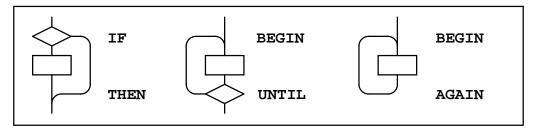
Figure A.1 – The basic control-flow patterns.
